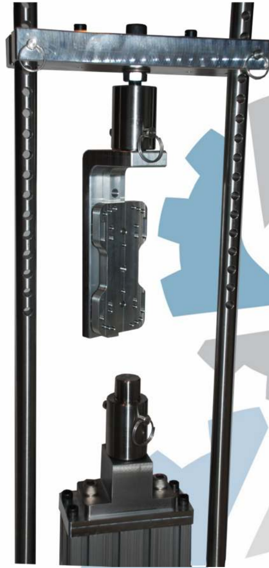
INVERTED orientation in PMLD-5000XLT
